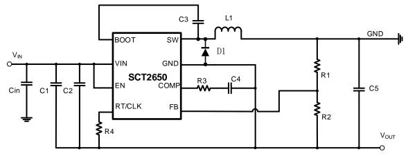
Figure 12. SCT2650 Inverting Power Supply
