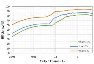
Efficiency, Vin=24V, Fsw=500KHz
