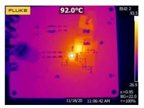
Figure 24. Thermal, 24VIN, 3.3Vout,5A
