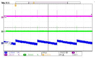
Figure 21. Output Ripple (Iload=0A)
