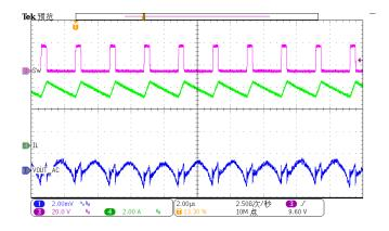
Figure 23. Output Ripple (Iload=5A)
