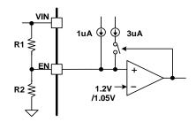
Figure 9. System UVLO by enable divide
