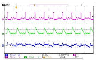
Figure 22. Output Ripple (Iload=100mA)
