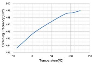
Figure 6. Switching Frequency VS Temperature
