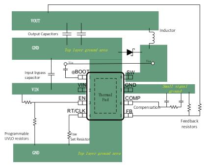
Figure 25. PCB Layout Example
