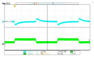
Figure 20. Load Transient (1.25A-3.75A, 1.6A/us)
