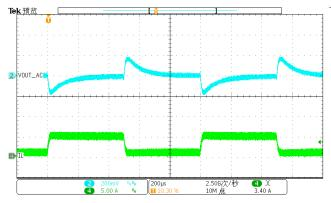
Figure 19. Load Transient (0.5A-4.5A, 1.6A/us)
