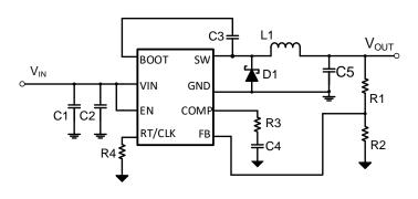
4.5V-60V, Asyncronous Buck Converter
