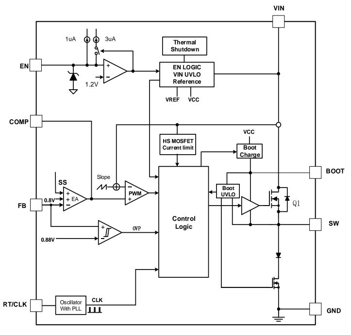
Figure 8. Functional Block Diagram
